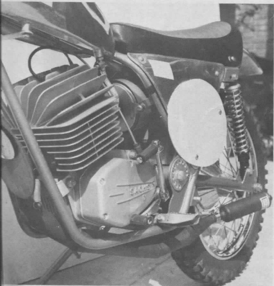
BELOW: Massive engine finning assures adequate cooling. Forward facing air inlet can mean trouble in deep water.
