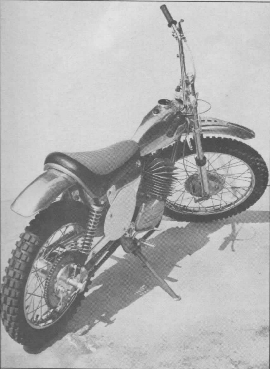
BELOW: Massive engine finning assures adequate cooling. Forward facing air inlet can mean trouble in deep water.
