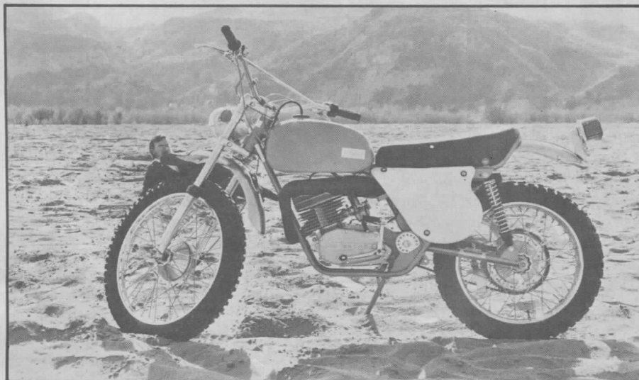
A P.C. Enduro prototype. Production model will have plastic fenders, different seat, possibly different suspension and VDO speedo.
