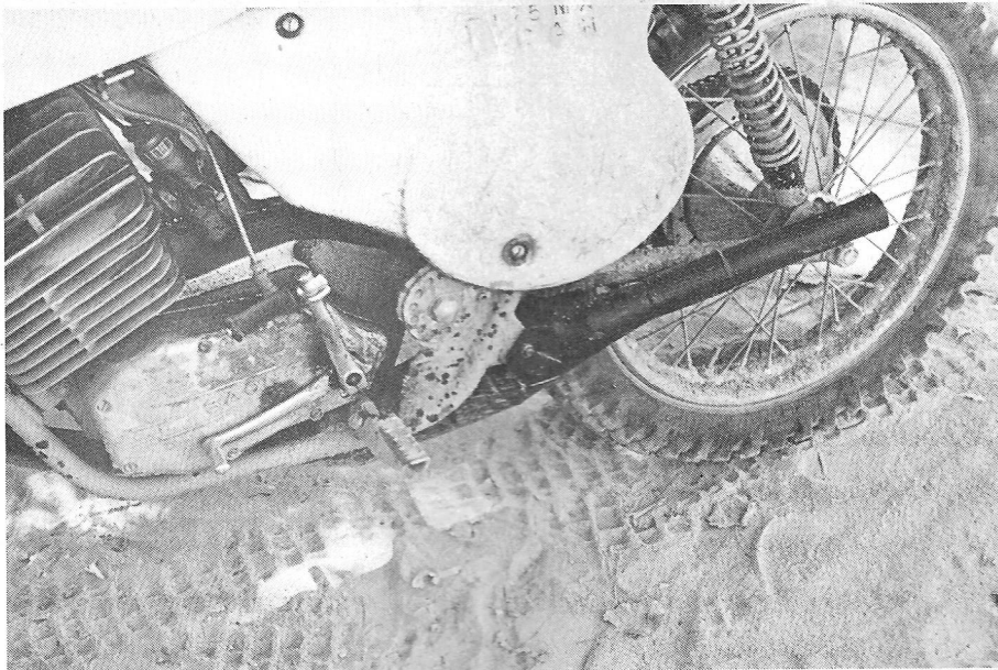
The English frame uses cams at the swingarm pivot to adjust the chain.
