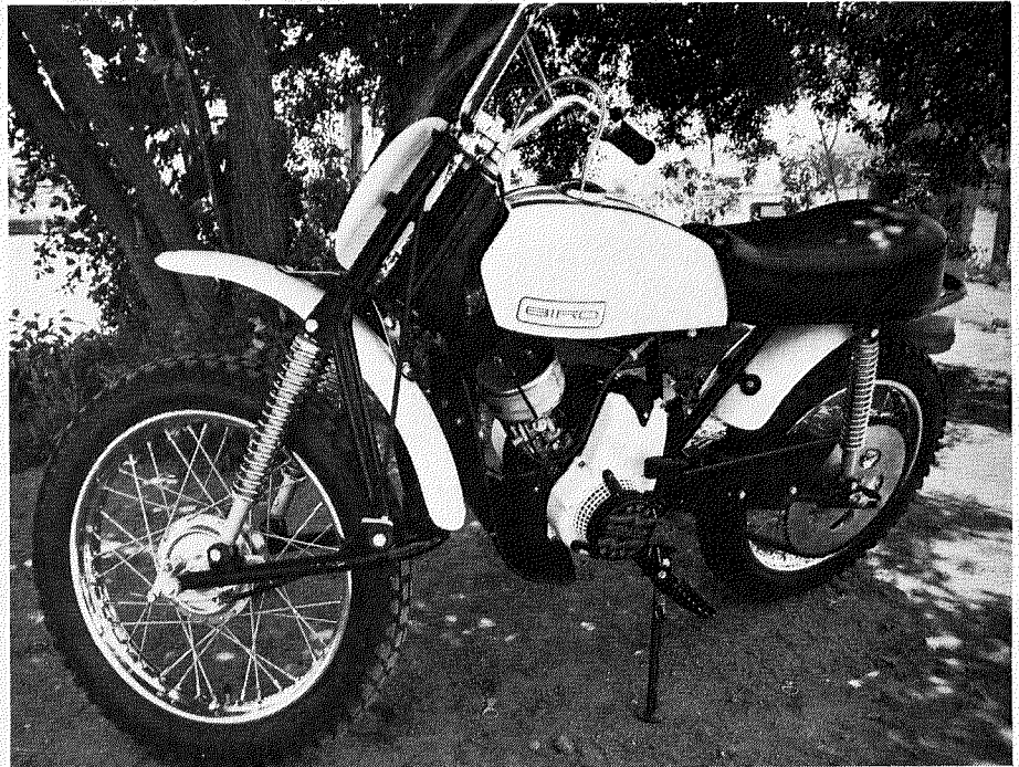
The Bird MX looks a bit unusual to the untrained eye because of the Mac engine and torque converter.
