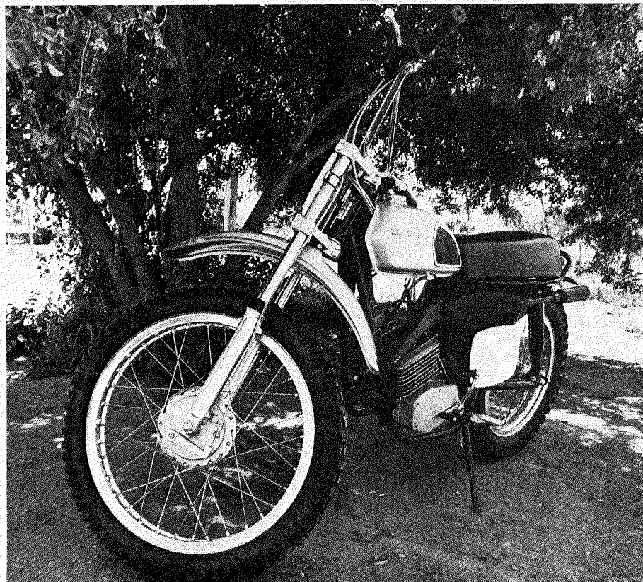
Front forks are Ceriani type and rims are Akront type. The choice of tires are German made Metzlers. Both fenders are unbreakable plastic.
