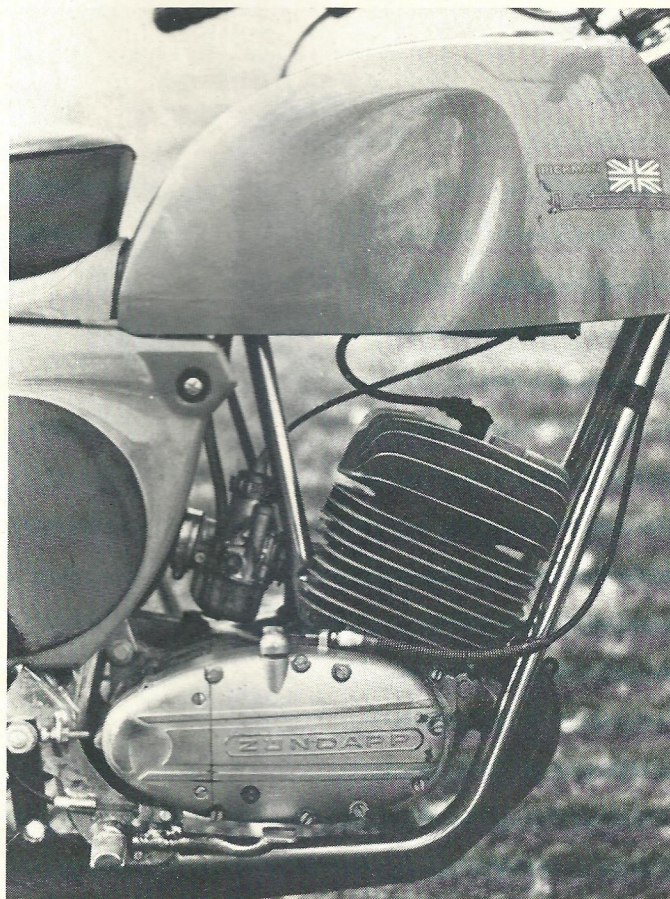
The Zundapp 125cc engine sucks up to 1.7 gallons of pre-mix per tank through the Bing carburetor. First kick starts are the rule.
