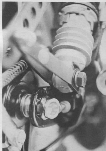
At full stroke the shock bangs into the axle and a spacer must be placed on the shock shaft to limit travel.
