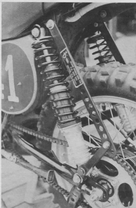
This is how it works. The swingarm and kit act as a double lever to multiply the stroke of the shock.
