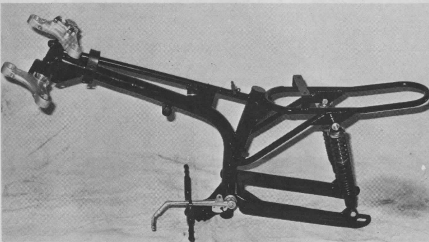
Six-inch wheelbase increase results from sections added to top tubes and longer swingarm.
