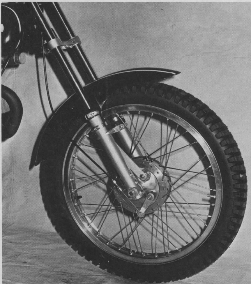
Because Ceriani forks are narrower, some work on hub was necessary. Fender by Rickman.
