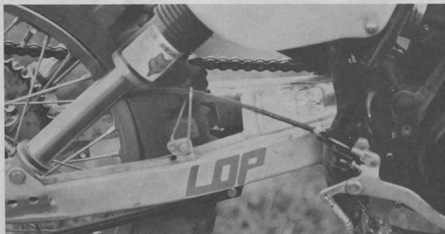
A pair of 17½-inch Fox Airshox did it all on the back end.
