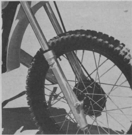
Al Baker kitted forks offer one full inch longer travel than stock.
