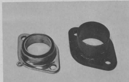
For more efficient breathing, the larger exhaust flange at right is used in conjunction with the triple-staged downswept pipe.
