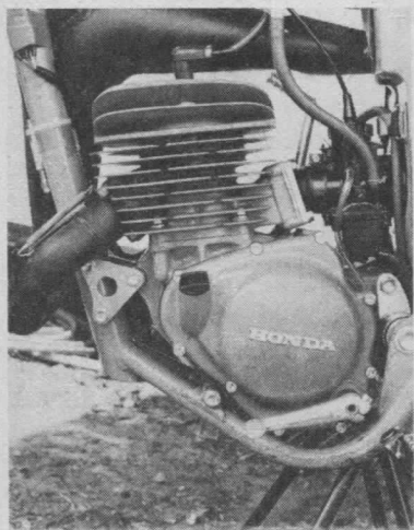
The left side of the latest RC works engine. Mill uses cylinder reed induction and gearbox now has six speeds instead of five as on the stocker.
