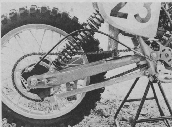
Close up of the aluminum swingarm and 17.5-inch AirShox kit on Wise's bike. Kit is available generally from Moto-X Fox.
