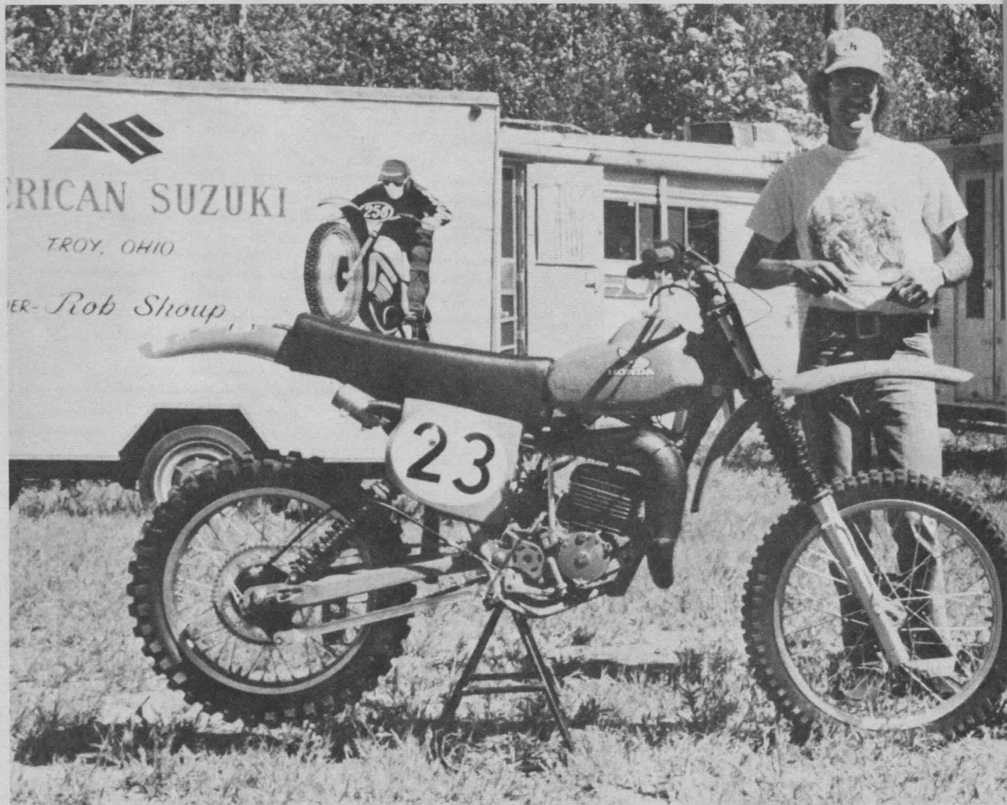
The left side of the latest RC works engine. Mill uses cylinder reed induction and gearbox now has six speeds instead of five as on the stocker.
