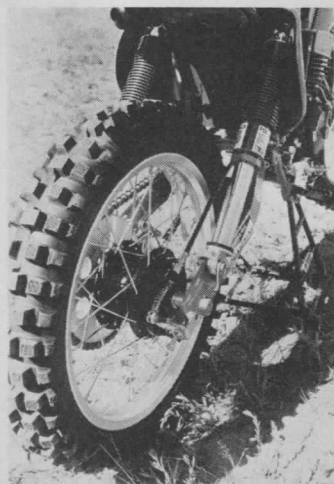
Close up of the aluminum swingarm and 17.5-inch AirShox kit on Wise's bike. Kit is available generally from Moto-X Fox.
