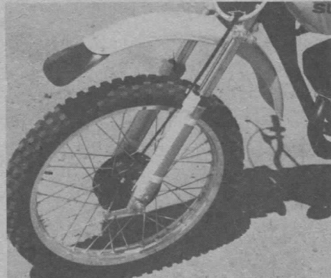
The one weak point on the Suzuki: the softly sprung front forks. The front suspension is no match for the rear on the stock machine.
