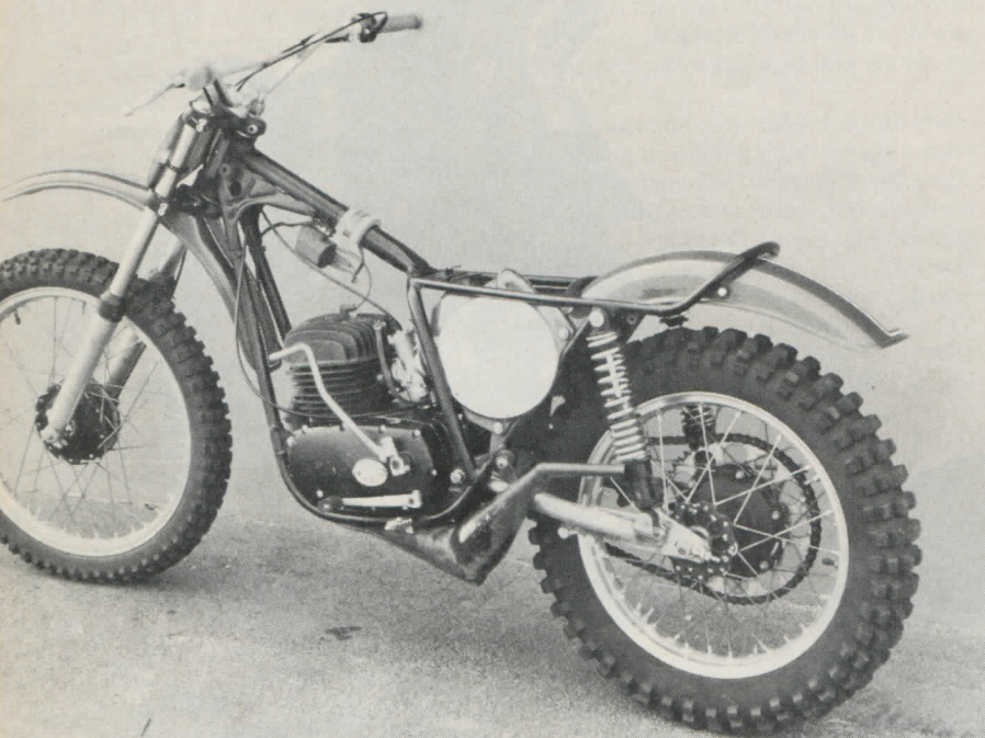
The double-downtube chromoly frame and aluminum swingarm keep the Phantom chassis light, and excellent Betor forks and well-engineered steering geometry make it one of the finest handling motocrossers available.
