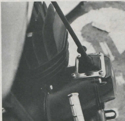
The carb sticks out the right side, like a rotary is supposed to; the button in front of the cable is the choke.
