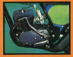
Carburettor, 36 mm Ø Bing Carburettor, wide power range, excellent torque.
