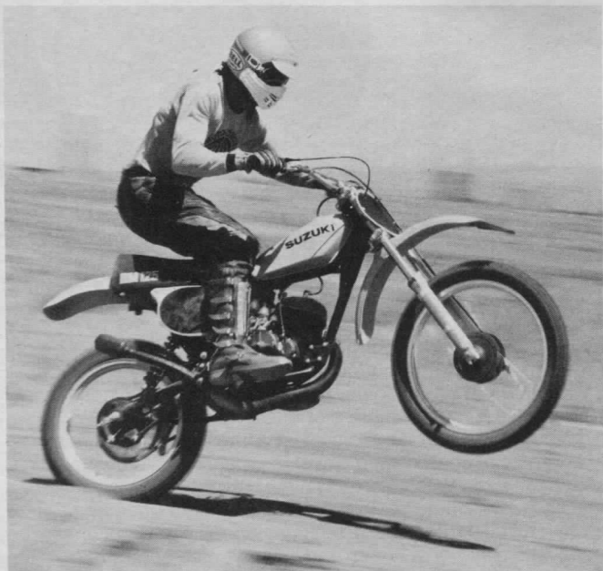
Long travel shocks may be seen at work in these two photos. Note distance between wheel and fender at full extension (left) and full compression (right).
