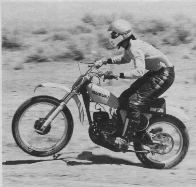
Long travel shocks may be seen at work in these two photos. Note distance between wheel and fender at full extension (left) and full compression (right).
