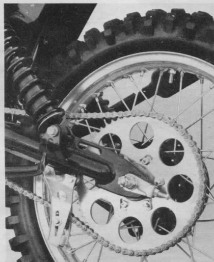
Forward mount shocks (above) result in 7.80 inches of rear wheel travel. Shocks are mounted upside down (left) so only the weight of the piston and damper rod is unsprung. Nitrogen is used inside gas/oil shocks instead of air because air corrodes.
