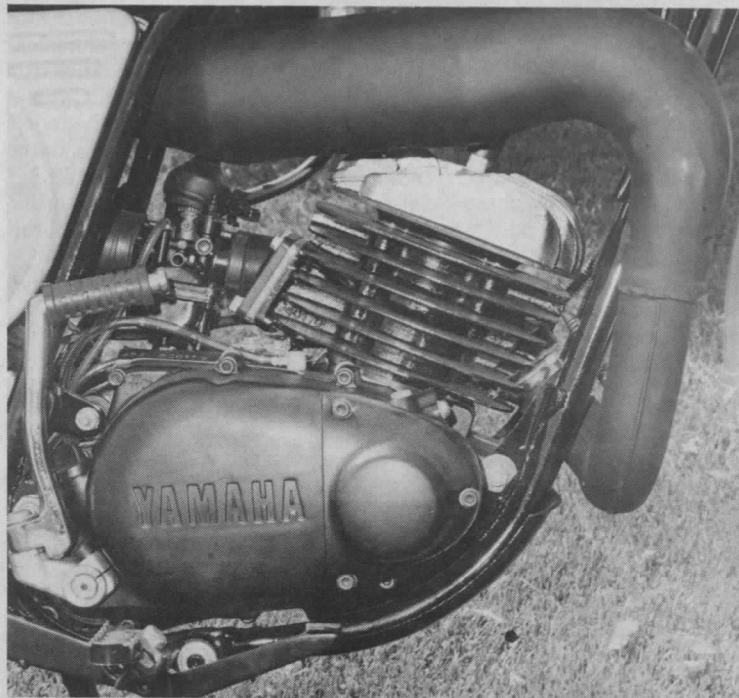
Reed valve engine does nothing sudden. The power though, peaks at an incredible 11,000 rpm.
