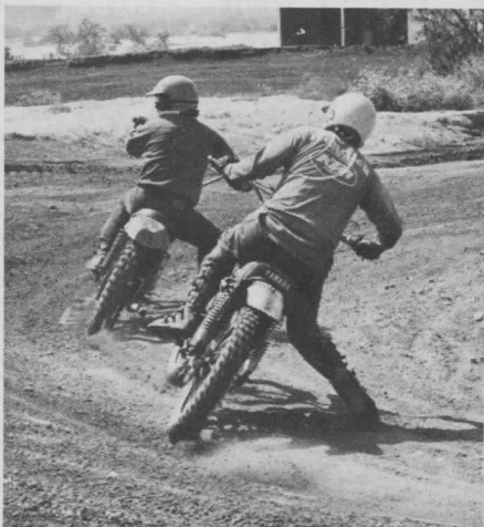
Wretched knobbies allowed rear end to wiggle out under power—like this.
