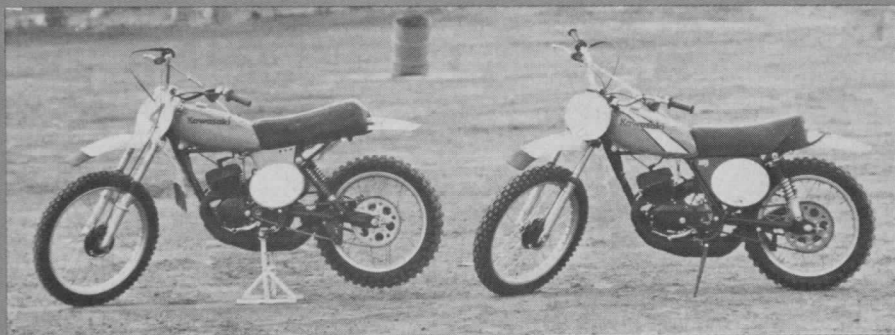
The stock KX-125 (right) and Jeff Wecker's modified machine. Aside from careful jetting and tuning on Wecker's racer, the engines are identical. The major modifications are in the suspension department.
