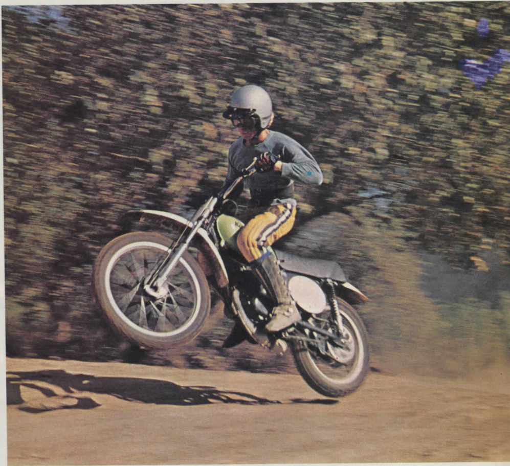
The aluminum-bodied rear shocks are light, but they look like they belong on a bigger machine. The tapered stinger/silencer on the end of the expansion chamber doesn't keep the KX125 quiet.
