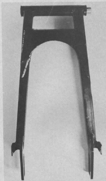
This swinging arm is a product of Red Line Engineering. It extends the wheelbase of the TM and will not flex like the stock arm. The one pictured is an early model. Production units will be nickel-plated.
