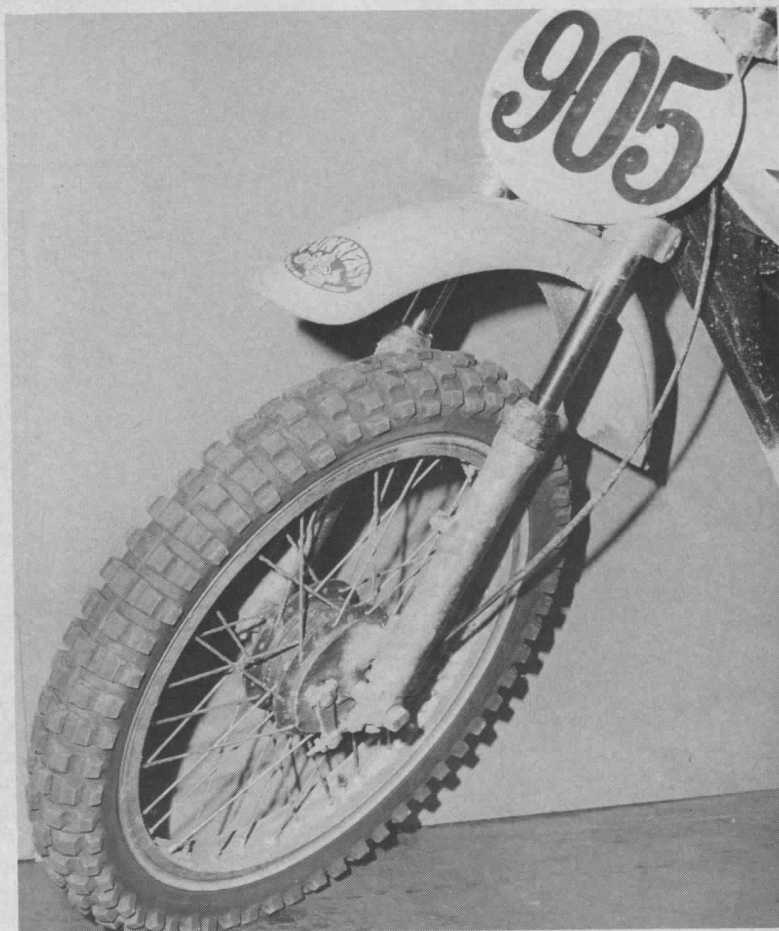
With the fork kit installed, the front end will treat potholes like they weren't even there. Yet, there is no externally noticeable difference between this manageable front end and a standard springy one.
