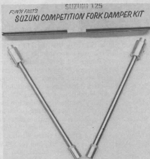
These two dampener rods from Fun 'n Fast, and 130cc of the proper weight oil, will transform the front forks of your TM into very well behaved units.
