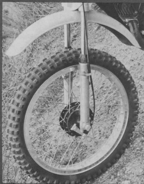
Slim-line Suzuki forks work well up to a point. That point being speed. Alloy rims help keep unsprung weight down.
