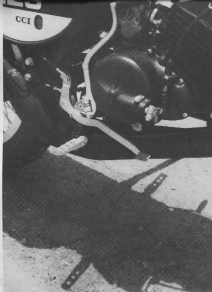
The brake pedal on the 125 is a metal strip with a small tab welded to the end. It is well-tucked-in, easy to operate, and in the event of a spill would not break easily.
