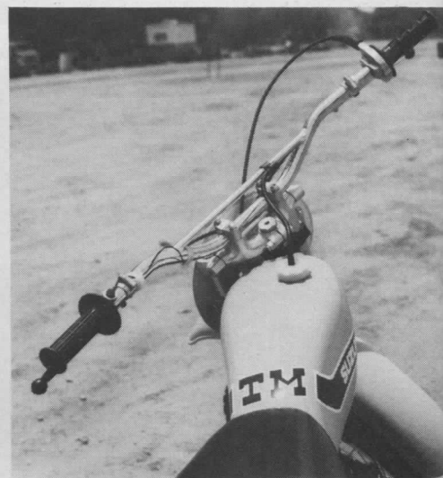
The handlebars are as spare as you could ask for. The kill button can be found on the left side. Note the slim tank.
