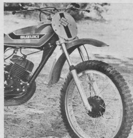
21-inch front wheel plus plastic everything make the Suzuki ready for fast riding and occasional crashing.
