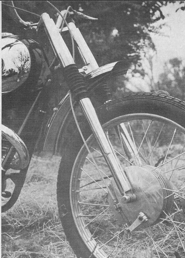
The chrome forks are set off by rubber dust covers but do not have enough travel for the rider who is serious about fast motoring.
