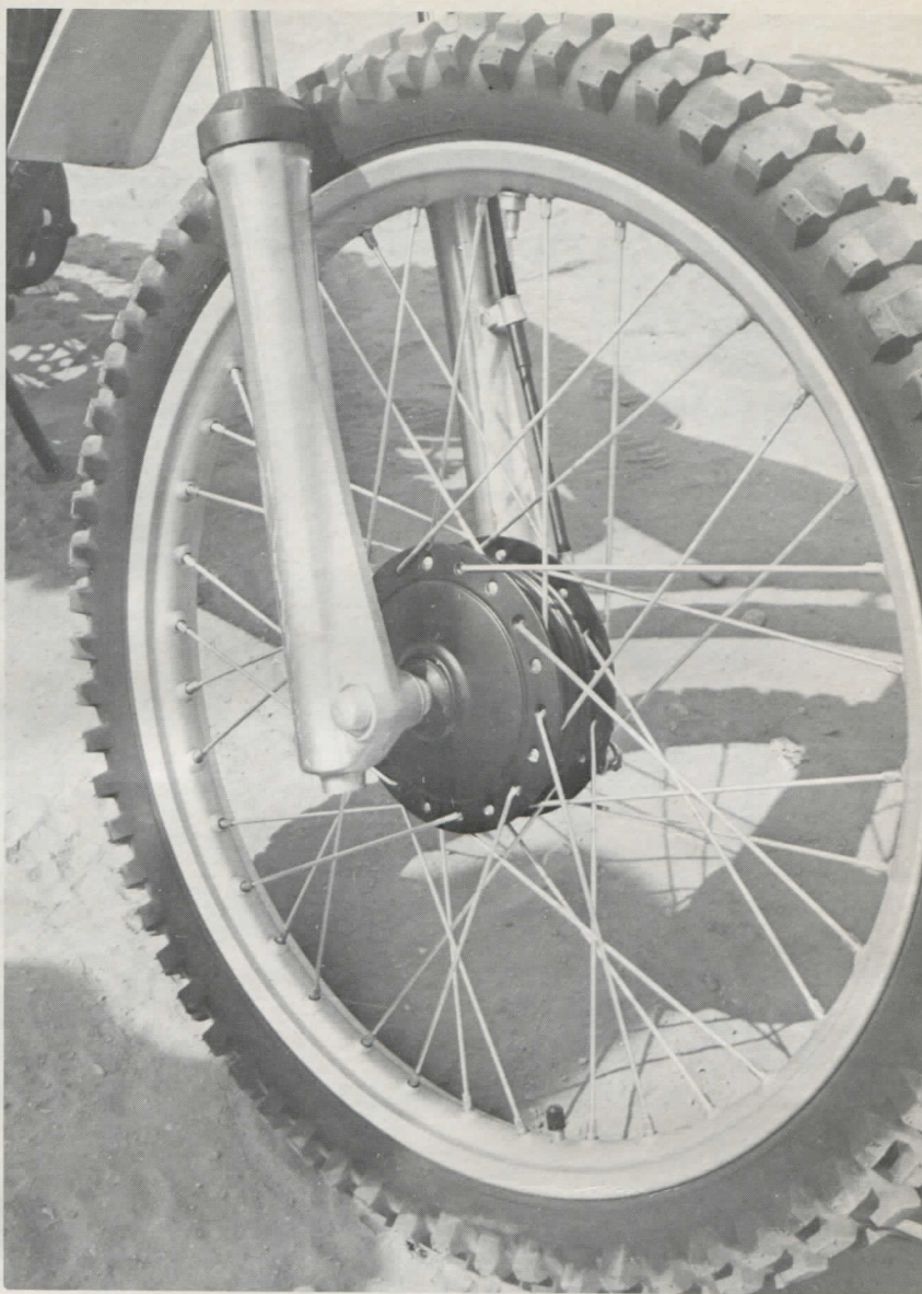
Front axle mounts forward like Bultaco enduros. (Thought we were going to say Maico, didn't ya.)
