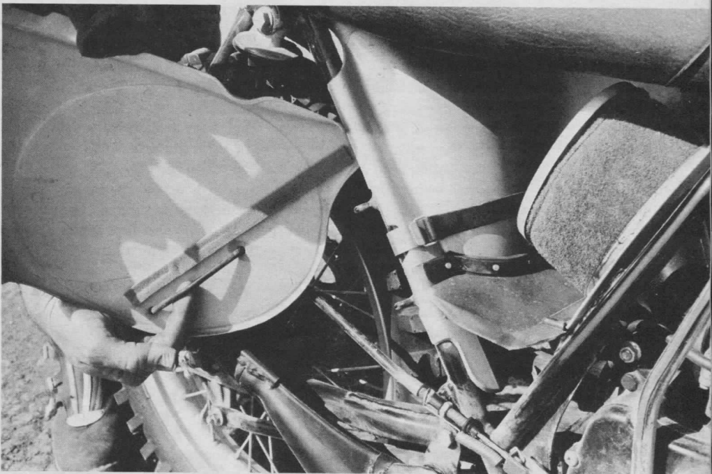
The plastic number plates and rear fender form sides of air cleaner box. Rubber bands hold on the plates.
