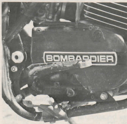
Brake lever sits way too high. A wire hook will pull it closer to toe level.
