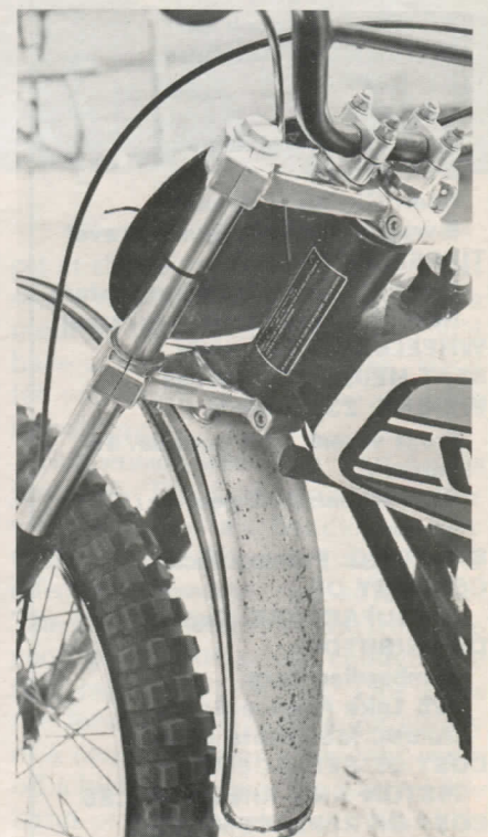
Eccentrics in the steering head allow rake to be changed by six degrees.
