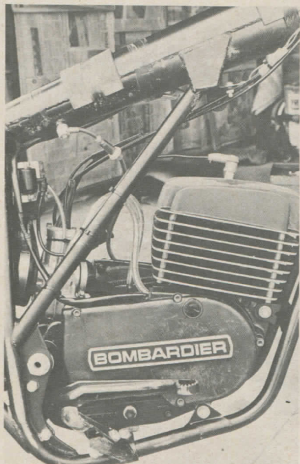
In the realm of the far-far out, check out the inline filter in the oil line coming from the top frame tube.
