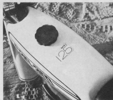
Wide plastic tank looked good, but got in way.
