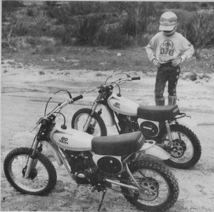
DG also makes a monoshock frame for the YZ-80. It too is quite a bit lighter than the stock unit.
