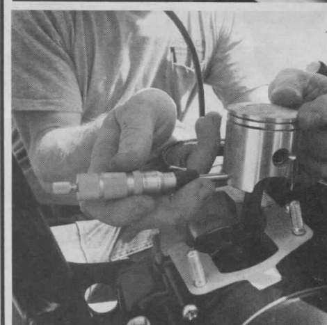
We measured the piston-to-cylinder clearance and piston ring end gap of all four bikes before and after the test to determine which one would wear out the quickest.
