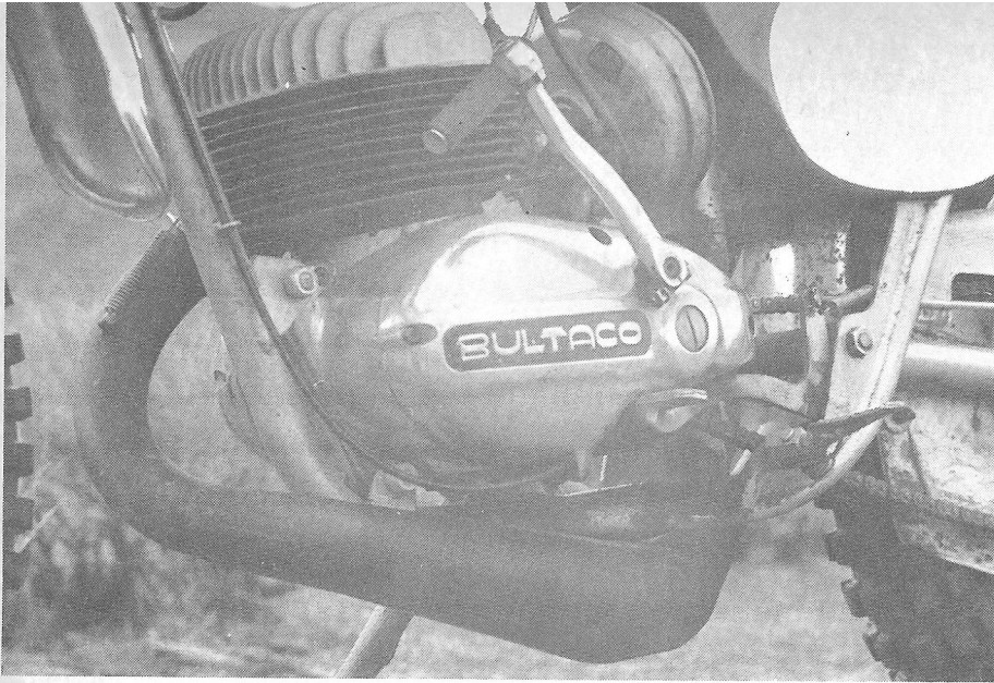
The 125cc engine shares its cases and transmissions with the bigger Bultacos. Exhaust is strictly dirt track.
