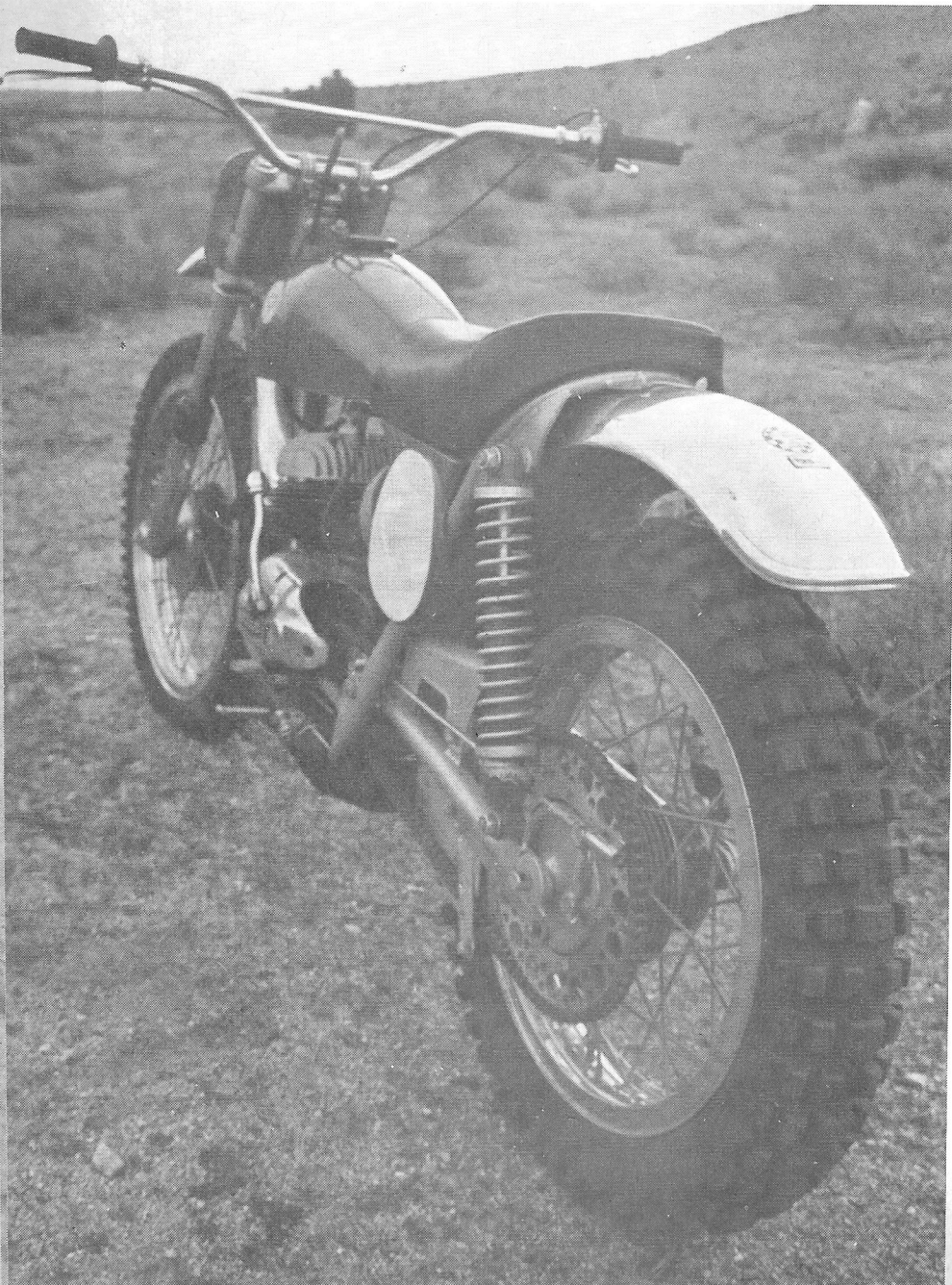
The 125cc engine shares its cases and transmissions with the bigger Bultacos. Exhaust is strictly dirt track.
