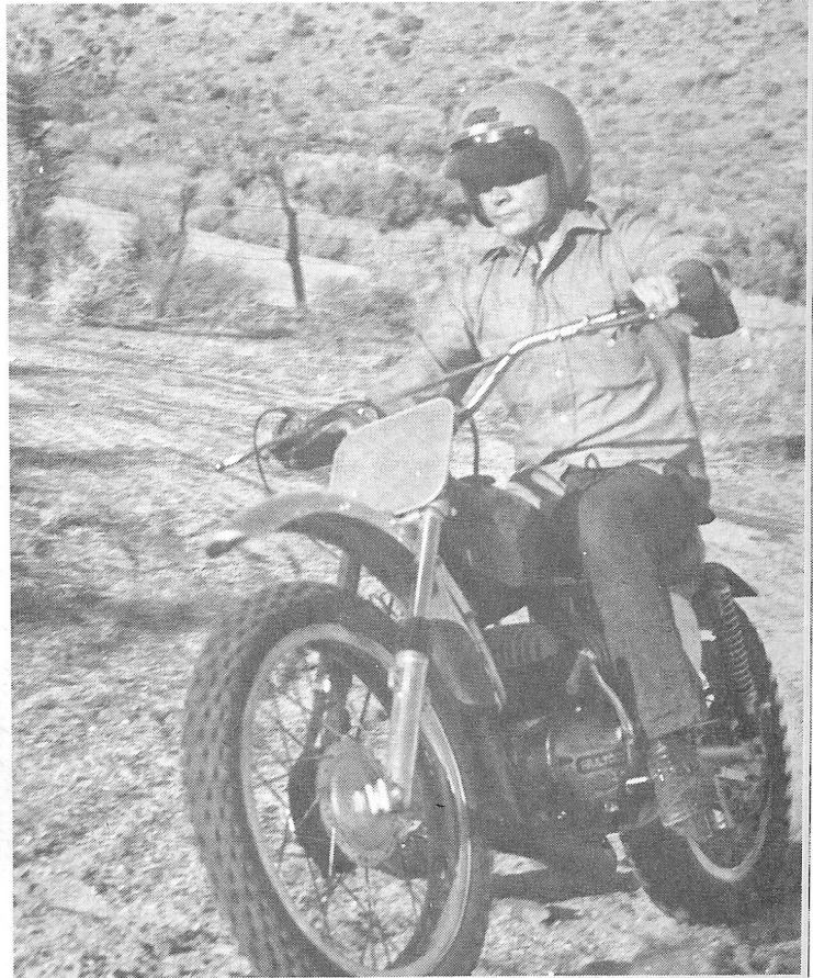
Seat position, peg location, and handlebar shape automatically place rider's weight in correct position for maximum control.
