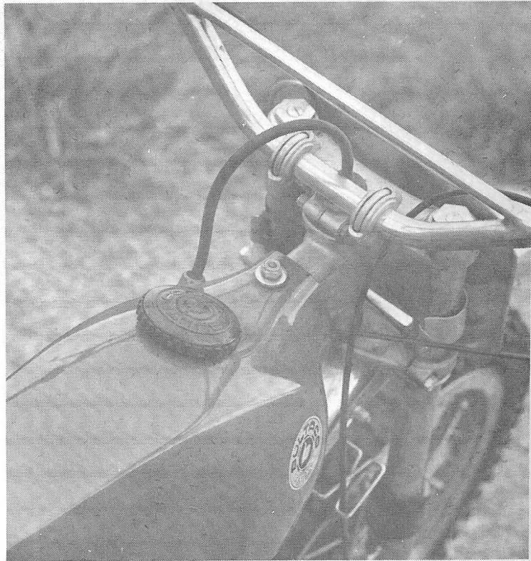
It would seem that no detail item has been overlooked as evidenced by the no-spill tank vent and one-bolt tank mount.
